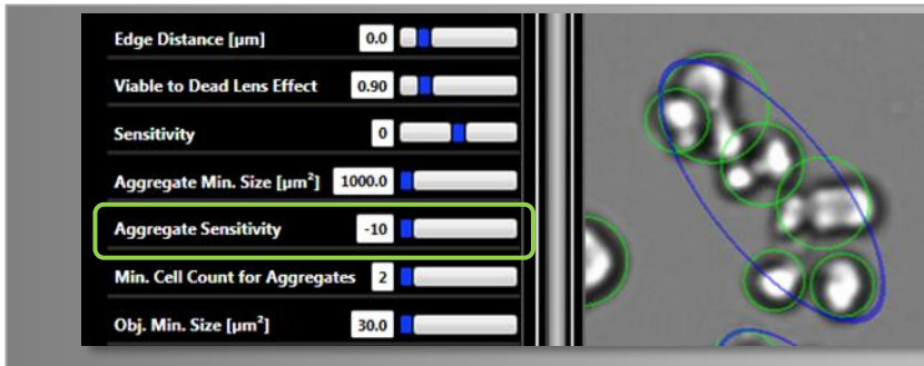
Fig. 19: Aggregate Sensitivity -10 6 cells are counted inside an aggregate.
