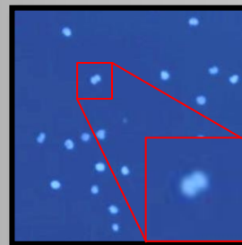
Fig. 6: Too bright. Decreasing exposure time or gain may help. Or modify staining protocol.
