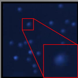
Fig. 4: Wrong focal plane. Signal from each nucleus is blurred and weak in contrast.
