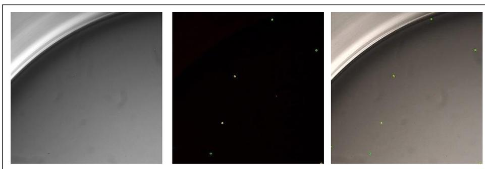
**Fig.1** Comparison of brightfield (left) and fluorescence (middle) images using CellTracker Red staining (at 2.5  $\mu\text{M}$ ). In the brightfield image the single cells cannot be detected. On the fluorescence image the small green circles indicate the detection of the single cells with the Cellavista software. The right image shows an overlay of both channels.
