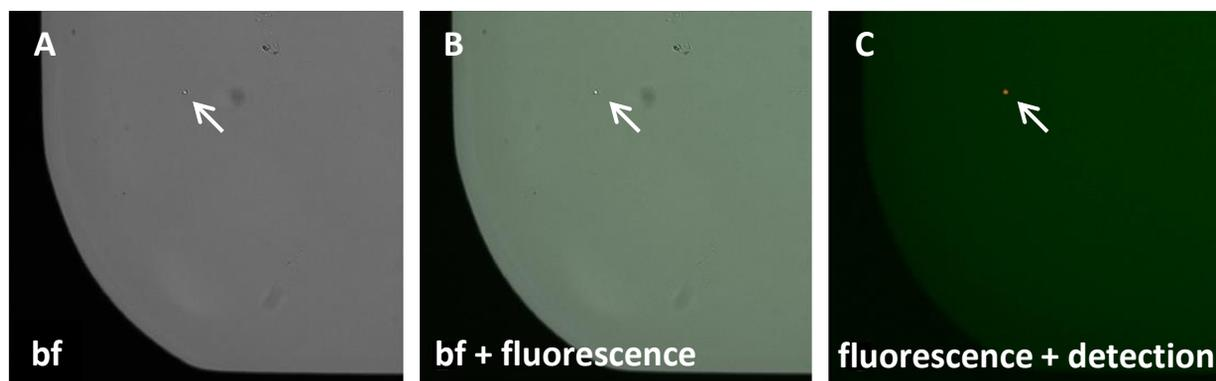
**Fig. 1 A-C: Automated detection of Calcein stained cells with the Cellavista System**
